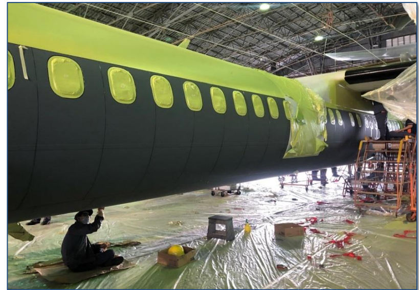
The sticking of the fuselage runway protective pad and the whole aircraft painting
