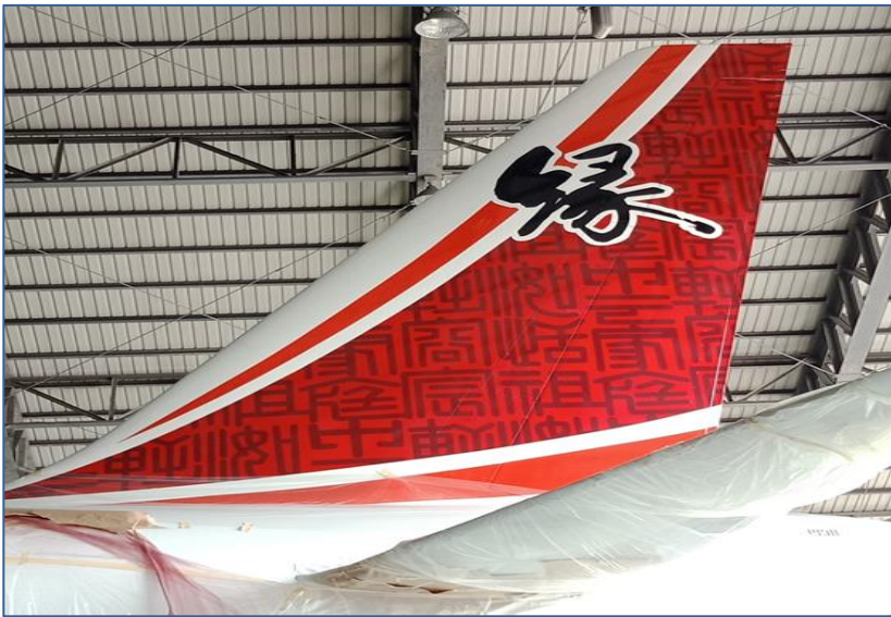
The exclusive pattern spraying of the straight tail fin of the customer's aircraft
